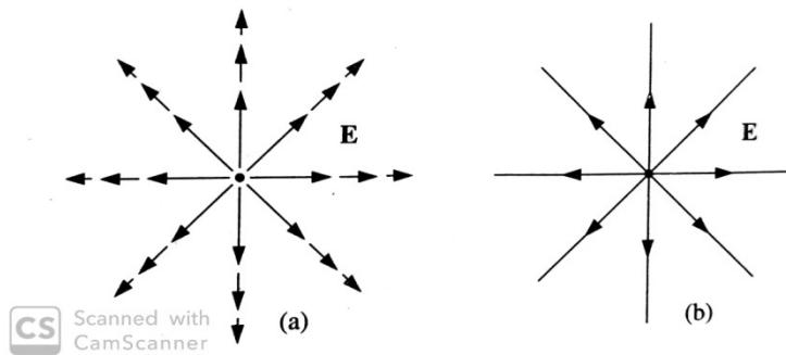
This vector function is directed radially outward and has a large positive divergence. This can be seen from the figure below.
